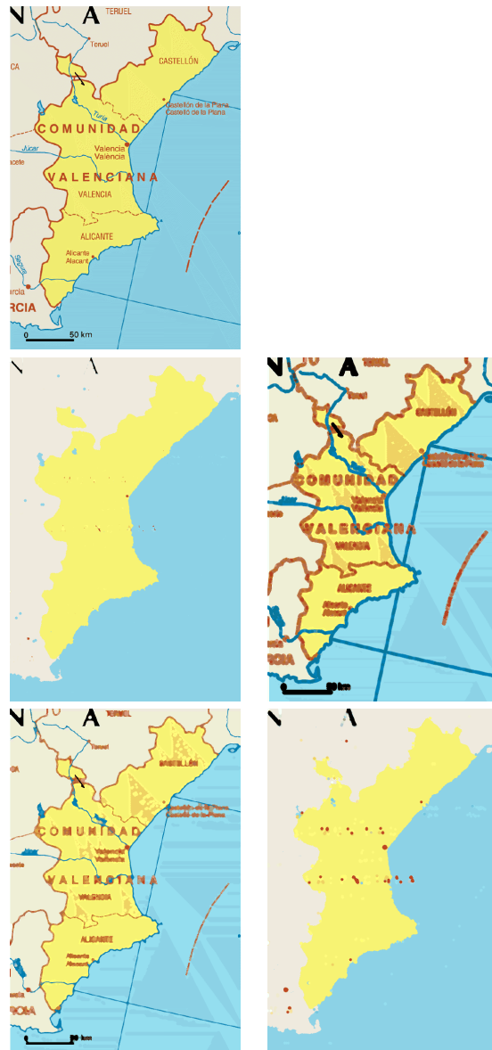
Figure 1: Valencia original map and erosion, dilation, opening and closing from left to right and up to down with a disk of radius 3 pixels. The RGB colour space and Mahalanobis distance has been used.
